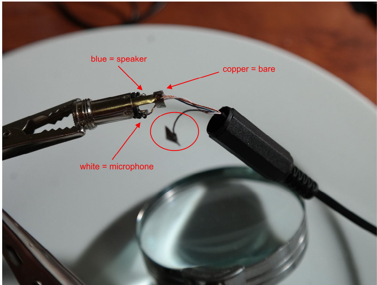
Figure 14: 2.5mm female jack with soldered XB1 chat cable wires.
