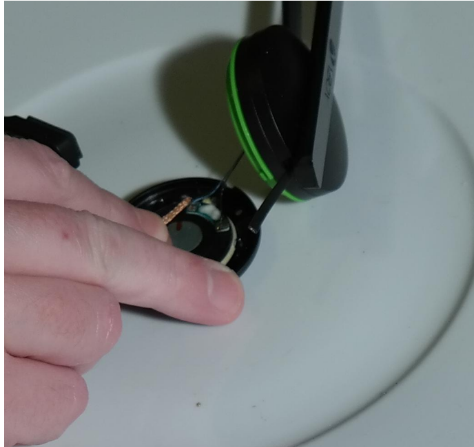
Figure 11: Desoldering of black and blue wires.
