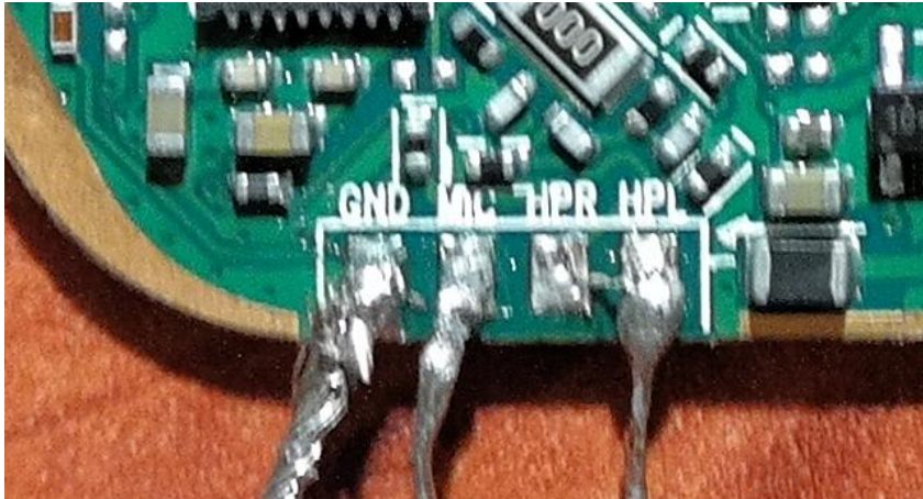
Figure 7: Original pin out (XB1 chat connector).
