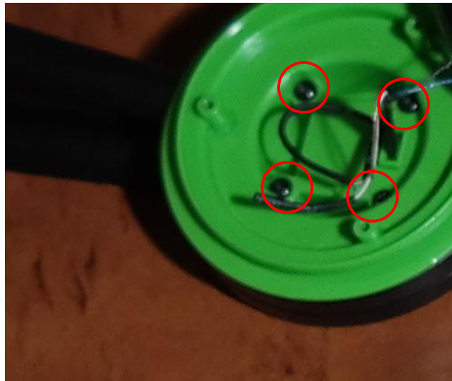
Figure 12: Four remaining TORX 5 screws.
