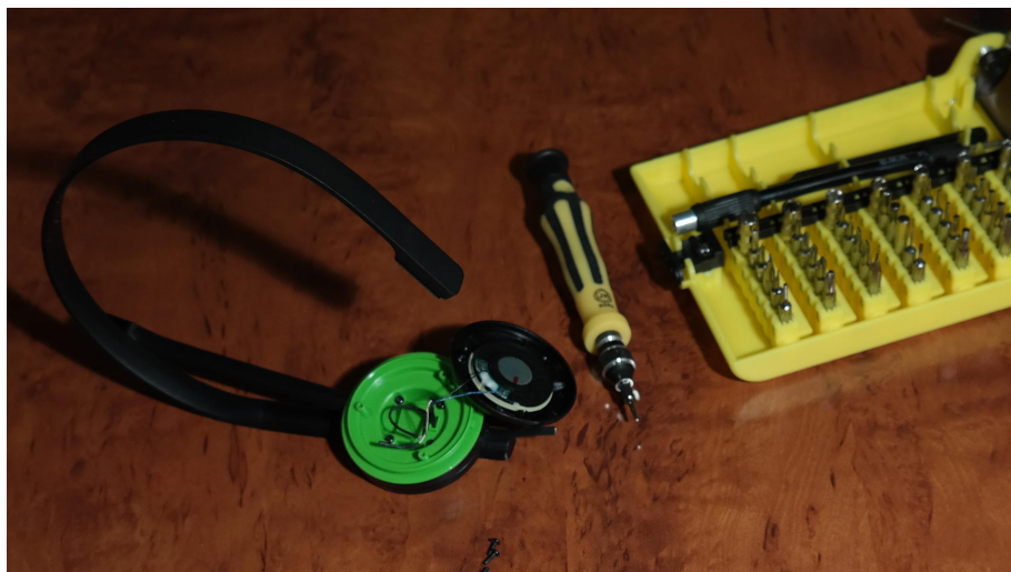
Figure 10: First three T5 screws removed, headset open.
