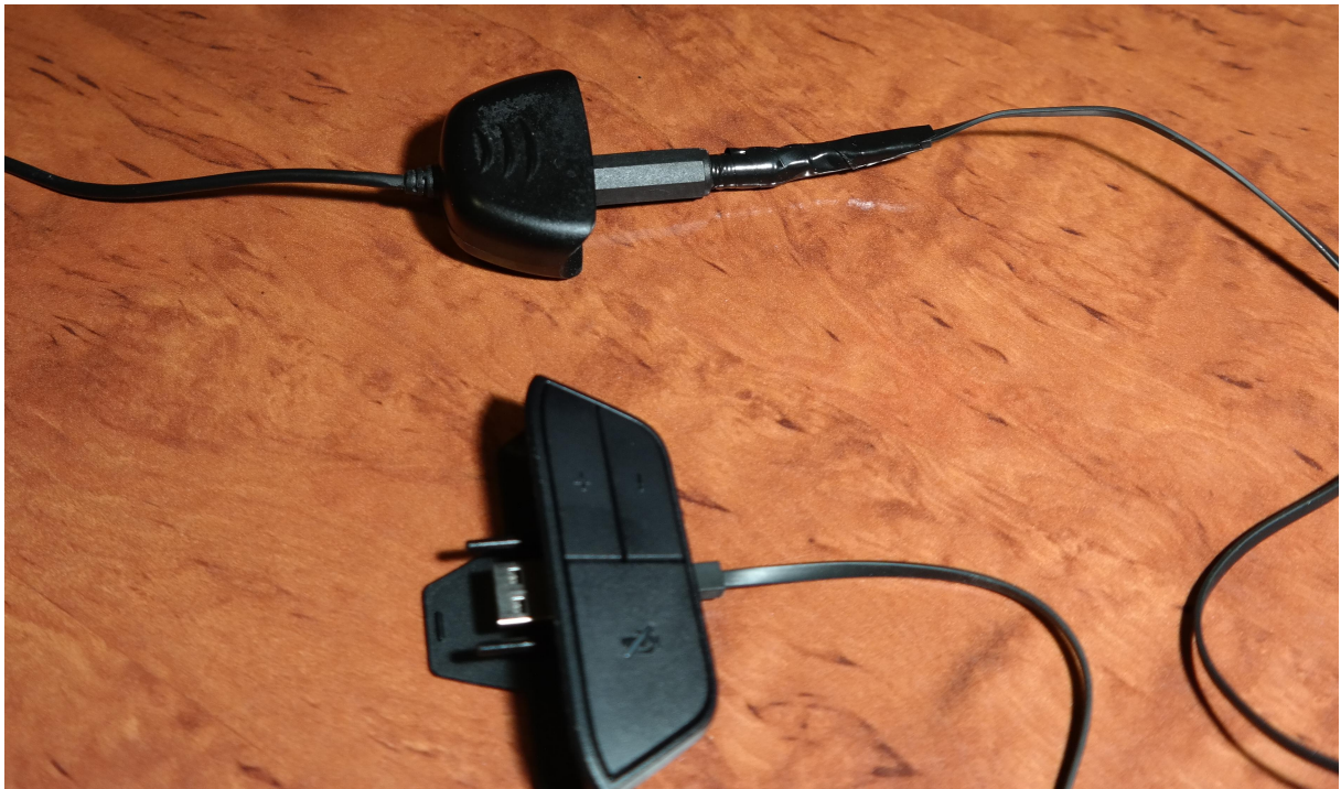
Figure 16: XB360 chat cable attached to XB1 chat cable.
